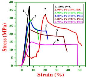
Figure 1: Pure PVC and PVC containing different weight percent of PEG.
