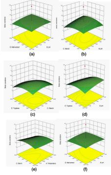
Figure 7:Response surface plots for the yield of  $\beta$ -carotene, changing components were malt extract and pH (a), starch and pH (b), tryptone and starch (c), tryptone and pH (d), starch and temperature (e), malt extract and pH (f).
