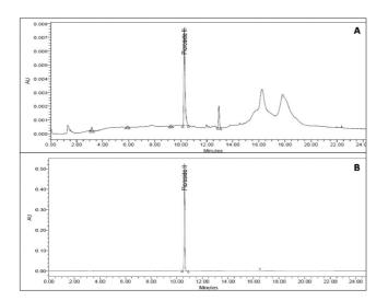
Figure 6 : HPLCchromatogram of A- in vitro cultureB- standard picroside-II at 265 nm
