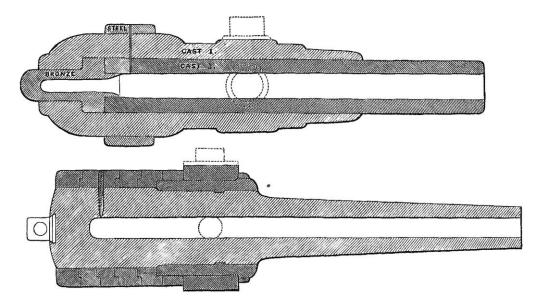
Figure 3. 11-inch Blakely gun probably sent in 1862, cast iron with steel hoops. And the 12.75-inch gun from Charleston. Blakely may have sent an improved version to St Petersburg. From Holley [1, p. 44]
