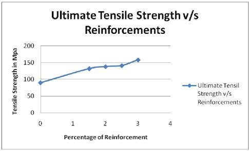
Figure: 3.1 Effect of graphite on Ultimate Tensile Strength.
