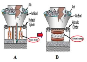
Fig.2: Ash bowl arrangement with (A) Guide roller and (B) Thrust bearing
