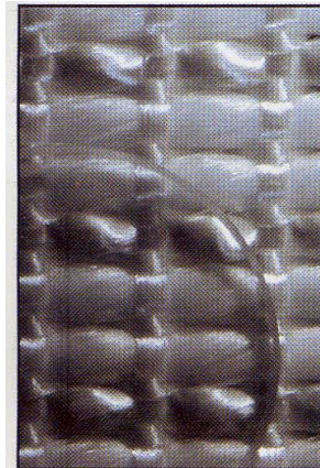
Fig. 6: show SEM of straight warp weaves.
