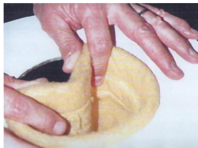
Fig.17: installing the bag into the tube sheet.
