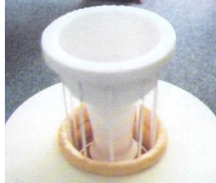
Fig.20: Cage being installed into a bag.
