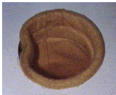
Fig.18: Incorrectly installed bag.
