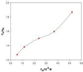
Fig.7. Langmuir isotherm of the adsorption of MB on Gypsum, Gypsum=0.025g, contact time 60 min, pH=6.0, temperature = $25^{\circ}$ C.
