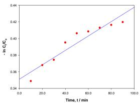
Fig.11. A plot of  $ln[C/C_o]$  vs. Time(t) for the First order reaction at room temperature
