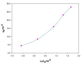
Fig. 9: Tempkin isotherm of MBadsorption On Gypsum, Gypsum= 0.025 gm, [MB] = 2.0×10-5 M, contact time 60 min, pH 6.0,
