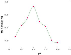
Fig.3. Effect of pH on MB adsorption on gypsum [MB]  $=2.0\times10^{-5}$  M, Gypsum=0.025 g, contact time 60 min, at room temperature.
