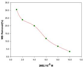
Fig.6. Change in adsorption of Methylene Blue on gypsum with its concentration, amount of gypsum = 0.025 g, contact time = 60 min, pH 6.0, temperature = $25^{\circ}$ C.
