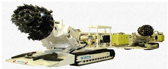
**Figure 6: Road Header Machine** Source: Mining Techonology.Com (2010)
