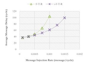
Figure 3: Average Message Delay (AMD) of FTR and i-FTR routing algorithms. 10% of faulty links with Hotspot traffic.
