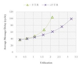
Figure 5: Performanceof FTR and i-FTR routing algorithms. 10% of faulty links with Hotspot traffic.
