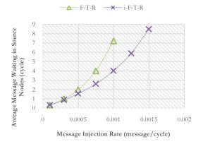
Figure 4: Average Message Waiting in Source Nodes (AMWS)of FTR and i-FTR routing algorithms. 10% of faulty links with Hotspot traffic.
