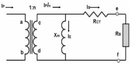
Fig. 1 Simplified equivalent circuit of CT
