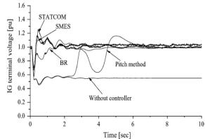
Fig. 7.Responses of IG terminal voltage.
