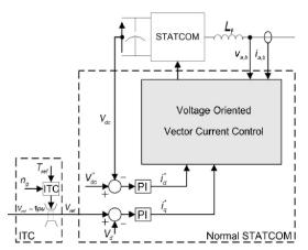
Fig 2. Proposed control structure of the STATCOM with ITC
