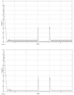
Fig.4 (a) Torque oscillation with grid fault (period 1.5 sec -2sec) – Without STATCOM, (b) With STATCOM
