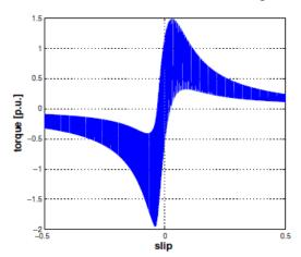
Fig1. Simulated torque-slip characteristic for a single-phase to ground fault (1ph  $\rightarrow$  0)
