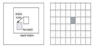
Figure 1: Block-Matching Motion Estimation [15]
