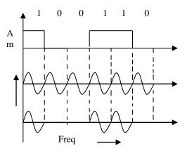
Fig.5: Amplitude Shift Keying
