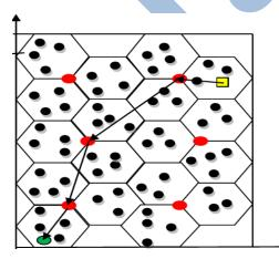
Fig 8 sink sends a query req. to the source
