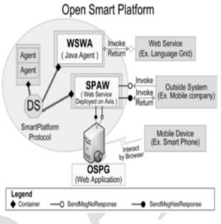
Fig: 1 Open Smart Platform architecture for single Smart Space
