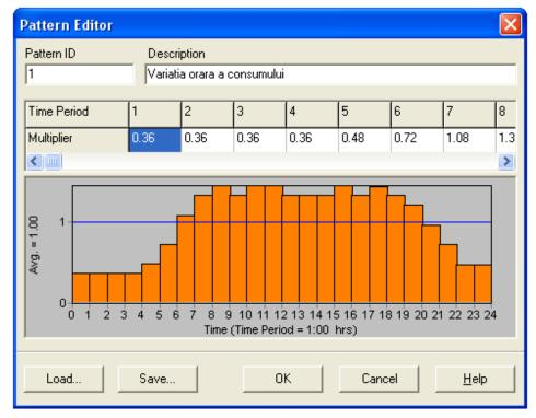
Fig.3. Hourly variation diagram for water consumption.
