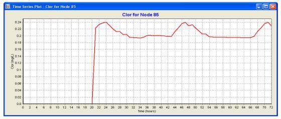
Fig.5. Residual chlorine concentration in junction 85 (Ohaba Strei).
