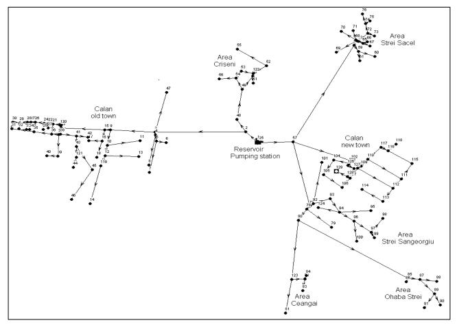
Fig.1. The diagram of the distribution system (the junctions and the service areas).
