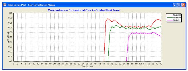
Fig.7. Variation of the residual chlorine concentration in Ohaba Strei area.
