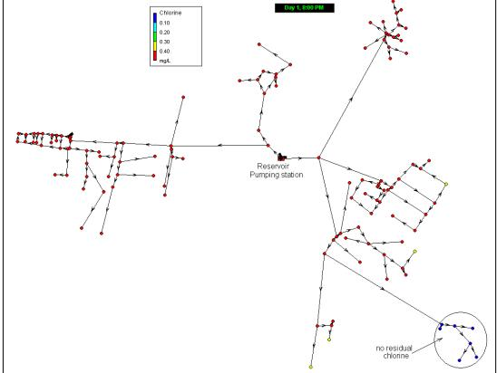
Fig.6. Residual chlorine concentration after 20 hours.
