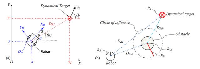
Fig. 1. (a) Attraction to a dynamic target and (b) The used perceptions for mobile robot.
