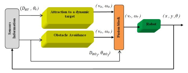
Fig. 5. The proposed control scheme.
