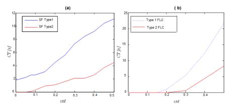
**Fig. 9**. Evolution of the Collision Time of the type-1 and type-2 FLC, (a) : gaussian MFs, (b) : triangular and trapezoidal MFs.
