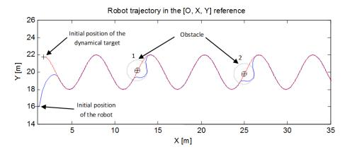
Fig. 7. Robot trajectory reaching a dynamic target (moving sinusoidally) while avoiding obstacles.
