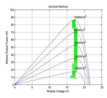
Figure 8. IncCond algorithm with various irradiations
