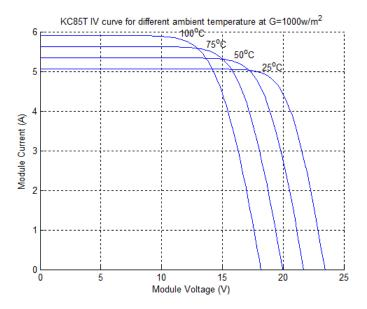
Figure 6. KC85T module I-V curve at various temperatures
