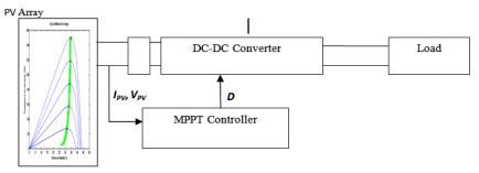
Figure 1. Photovoltaic system with MPPT
