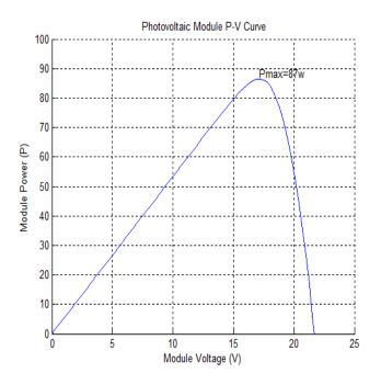
Figure 5. KC85T P-V curve.
