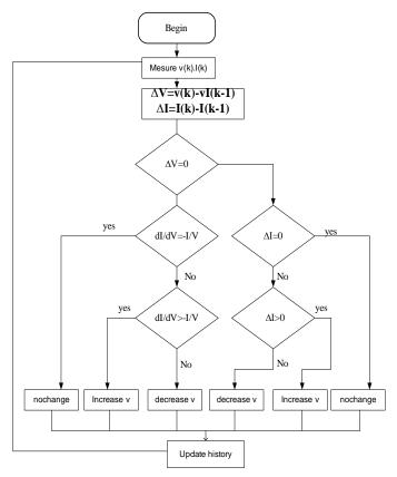
Figure 2. The flowchart of the InCon method
