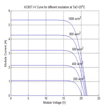
Figure 7. KC85T module I-V curve at various insolation.
