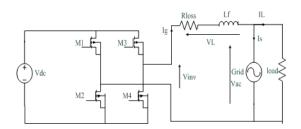
Figure 9. Full bridge grid connection.
