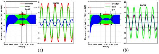
Figure 15. (a,d) Simulation shape of currents Igrid, Iinv and Iload.
