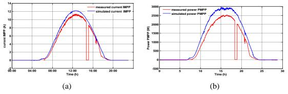
**Figure 7.** (a) Illustration the measured and simulated current, (b) Illustration the measured and simulated power.
