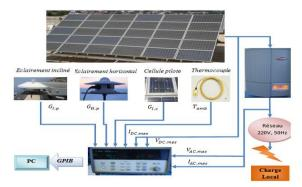
Figure 5. Synoptic total of the system acquisition.
