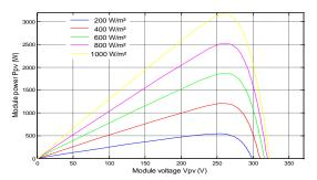
Figure 4. P-V characteristics of PV panel
