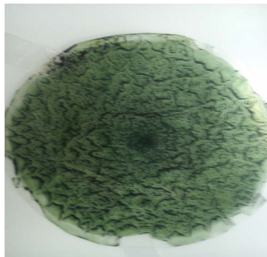
Figure 2. Natural look of the obtained film of polyaniline.
