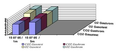
Figure 6: Comparison between express and chromatograph analysis of O2 and CO2 at Chisinau landfill
