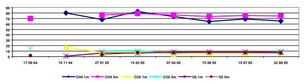
Figure 5: Dynamics of biogas measurement at Chisinau landfill
