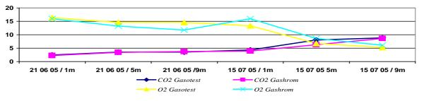
Figure 2: Comparison between express analysis and chromatograph of O<sub>2</sub> and CO<sub>2</sub> emissions at Strășeni landfill
