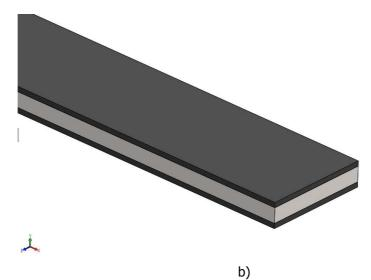
Figure 1. Laminated structures: a) three-layer beam and b) five-layer beam
