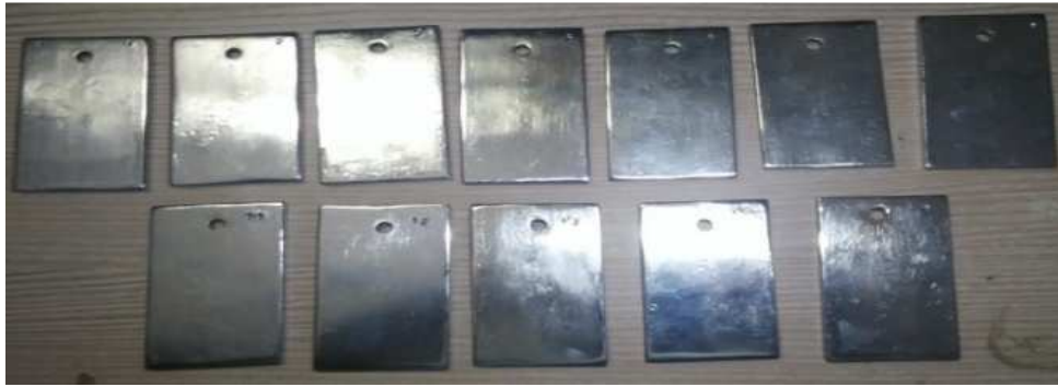
Figure 3.6: Specimen after Ni-Cr Plating
