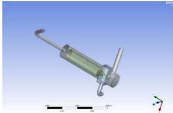
Figure 9: Complete Assembly of Float
