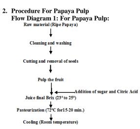
Raw material was obtain from local market, basic operation was done by manually like cleaning and washing of fruits then cut the fruit with help of knife and remove the seeds from fruit. Then cut into pieces and with help of pulper pulp will be collected in stainless steel pot. The pulp was pasteurised in stainless steel steam jacketed kettle and pulp was collect in stainless steel pot for further use and stored at 4°C temperature.
