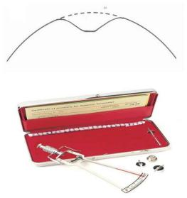
Fig 1: Corneal deformation in indentation tonometry (a); the instrument (b)
