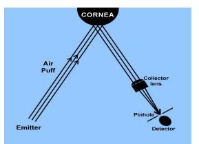
Fig 5: (a) Principle of Non-contact tonometer- emission of air pulse, (b) flattened cornea and reception of air puff
