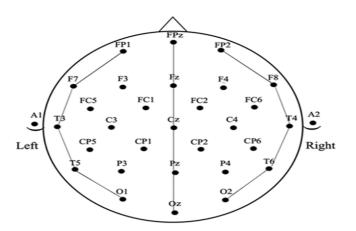
Figure 1: International 10-20 System for Electrode Placement Over Scalp
