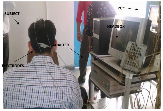
Figure 5: Experimental Setup for EEG Acquisition
