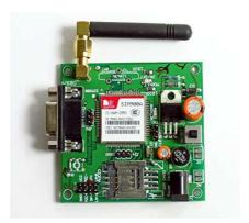
Figure 6: GSM Module
