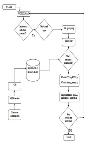
Figure 3 Basic design of the system
