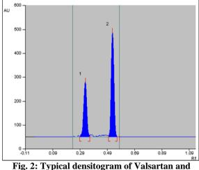
Fig. 2: Typical densitogram of Valsartan and Cilnidipine
