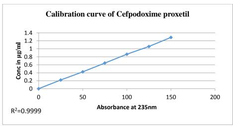
Figure 2- Calibration curve of Cefpodoxime using methanol.
