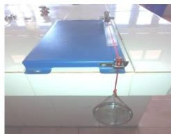
Figure.1: Modified instrument used for the measurement of tensile strength.
