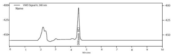
Fig 5: Specificity Sample chromatogram of Diltiazem HCl
