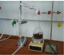
Figure- 2: Clevenger apparatus
