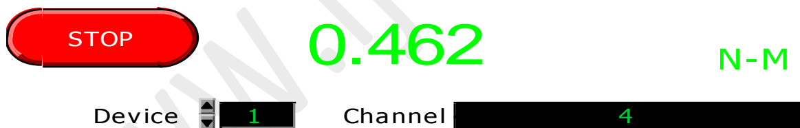
Figure 8: Torque output produced by Dynamometer expressed in terms of Newton Meter read from analog input channel #4
