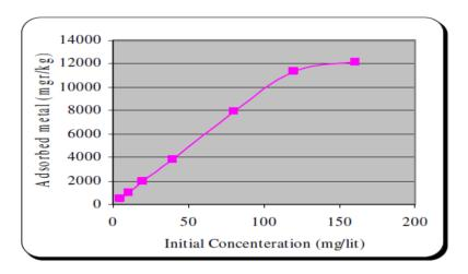
Fig. 8 Adsorption Isotherm for Analsim
