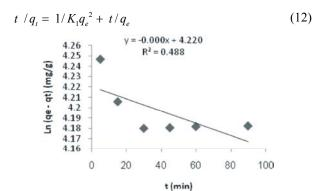
Fig 9: Kinetics data for first-order reaction
