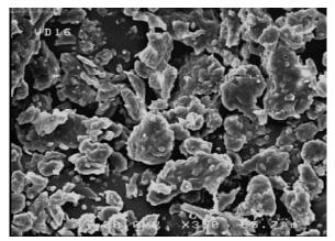
Fig 13: SEM image of the *Ziziphus nummularia* kernel adsorbent before adsorption
