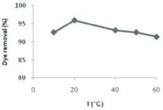
Fig 4: Effect of temperature on adsorption process
