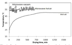
Fig. 4: Product temperature progressions during drying process
