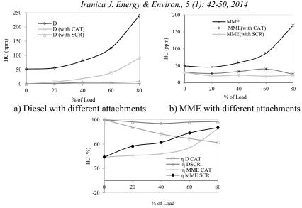
c) Conversion efficiencies of CAT and SCR with Diesel and MME
