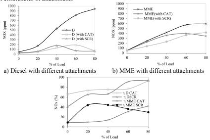
c) Conversion efficiencies of CAT and SCR with Diesel and MME
