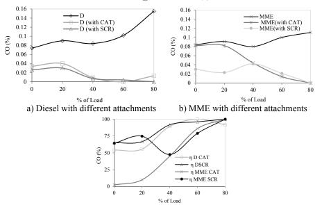
c) Conversion efficiencies of CAT and SCR with Diesel and MME
