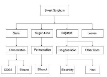
Fig. 2: Simplified diagram of Alternative Processes to Convert Sweet Sorghum to Energy Fuel
