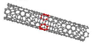
Fig. 4: Intramolecular junctions of third carbon nanotube
