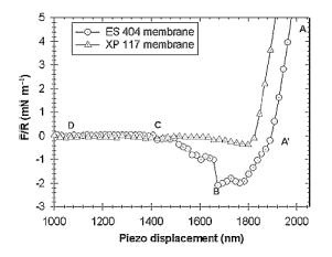
Fig. 3: Normalised retraction force versus displacement for a polystyrene colloid probe and two filtration membrane at pH 8.0, 10G<sup>2</sup> M NaCl.
