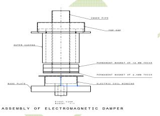
According to the Lorentz force law, the relative movement of the magnets and the conductor causes the eddy currents to induce in the conductor, producing the magnetic flux that opposes the external magnetic flux density, resulting in a damping force per each pole piece (Ebrahimi et al 2008b)
