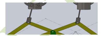
Fig12: Piston connection with link assembly
