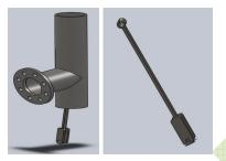
Fig14: cylindrical inlet housing piping and piston assembly.
