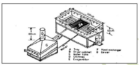
Fig. Diagram showing general features of drying
