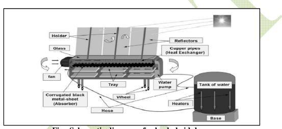
Fig. Schematic diagram of solar hybrid dryer
