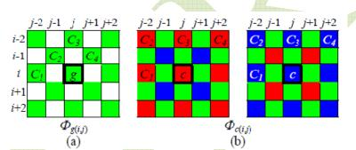
Fig4. The support region of (a) a green sample and (b) a red/blue sample
