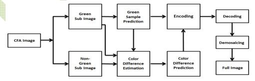
**Fig3. Structure of compression Scheme**
