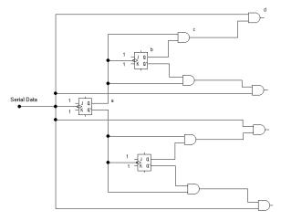
Figure 3: Serial to parallel converter circuit. High level voltage has been applied to all J and K inputs. All JKFFs have been worked as toggle FF.
