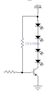
Figure 4: LED driver circuit.
