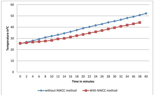
Figure4: Temperature variation of stator with and without NWCC method
