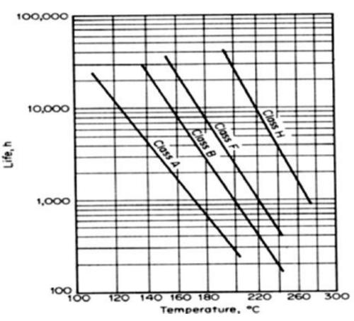
Figure 1. Insulation life versus temperature rise.
