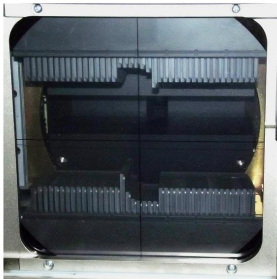
Fig. 7. Multileaf collimator (MLC)
